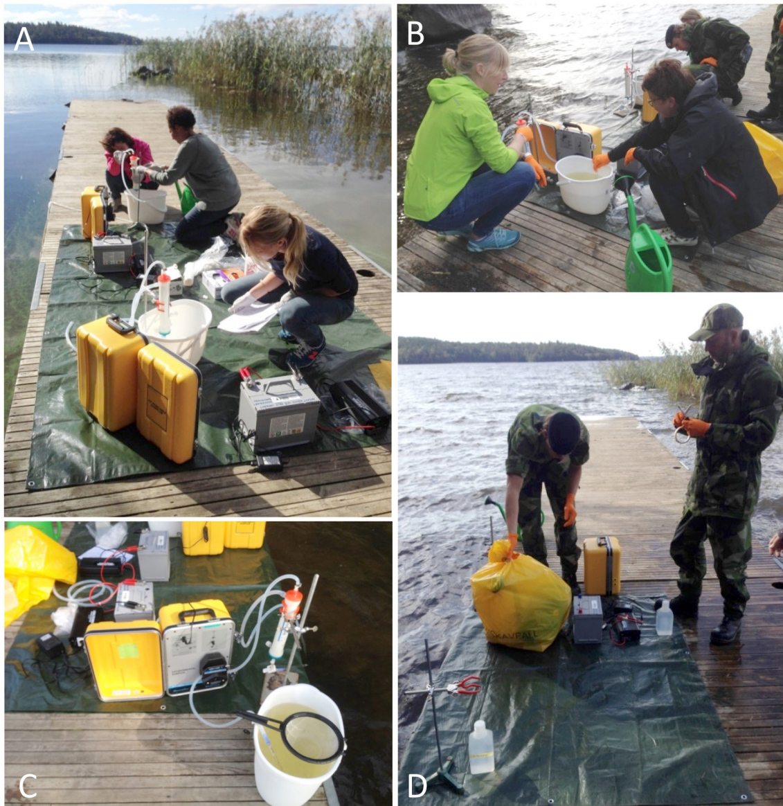
Figure 9. Panel A shows setup of sampling equipment at Mälaren. The portable pump (yellow) is powered by an RV battery (grey). The ultrafilter (with orange and blue ends) is mounted in a holder. A tarpaulin is used to demarcate the area where possibly contaminated water is handled. Panels B and C show the sampling. The water sample in the bucket is pumped into the filter and tubing leads the flow-through back into the lake. In panel D, the sampling has been completed. Most of the equipment has been repacked and all waste is put into a bag for contaminated material. Everything is brought back to the laboratory.
