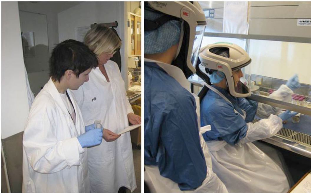
Figure 2. The two photographs illustrate differences in personal protective equipment in BSL2 (left) and BSL3 (right) laboratories. In the BSL2 laboratory, the staff wears lab coat. Gloves are only worn upon risk for contamination (of hands or sample). In contrast, the BSL3 staff wears a ventilated respirator powered by batteries in the belt, covering lab coat and soft boots, double disposable nitrile gloves, disposable sleeve protectors and apron. All work with the pathogenic microorganisms is performed within a safety cabinet.
